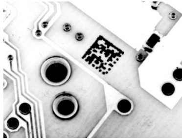
Figure 21 - Data Matrix Code Directly Marked on PCB Surface by Using Laser Etching Technology
