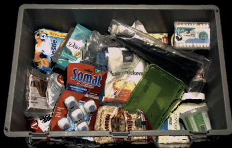
3D scan with color texture of mixed bin filled with transparent and glossy items
