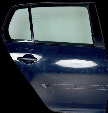
3D scan with color texture of car door, from 3,5 m / 11,5 ft
