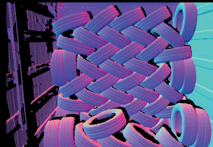
3D scan with normals showing a stack of black tires scanned from 4 m / 13,1 ft distance
