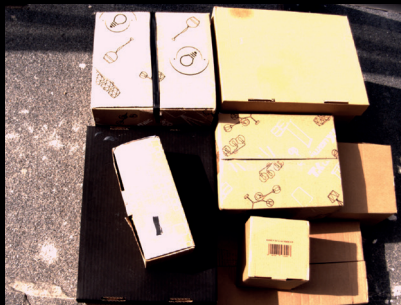
3D scan with color texture of boxes at high noon - 66ms capture time in dynamic mode
