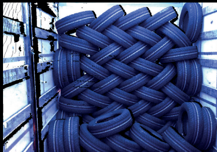
3D pointcloud with color texture showing a stack of black tires scanned from 4 m / 13,1 ft distance
