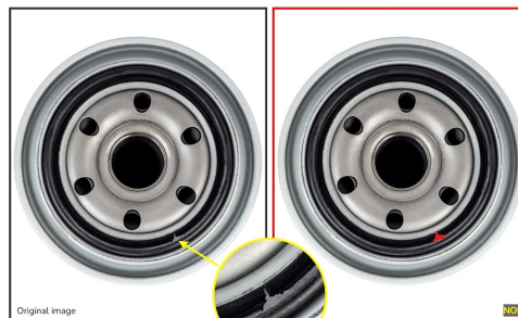
Oil filter quality Inspection
