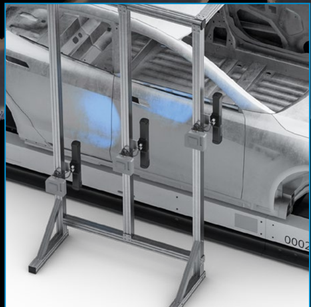
Gap and flush analysis in car assembly - ensuring seamless panel alignment and build quality.
