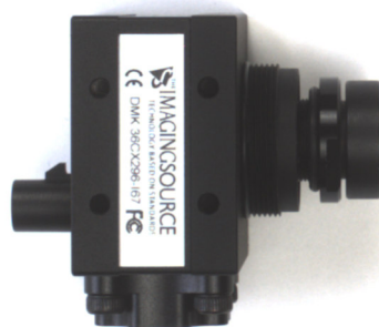
Figure 4: Camera with M12 S-Mount lens
