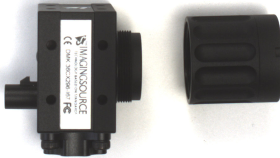
Figure 2: Unscrewed lens tube
